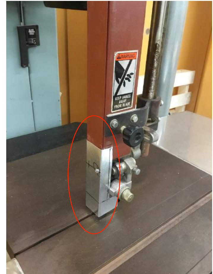
Bandsaw with additional guard.
