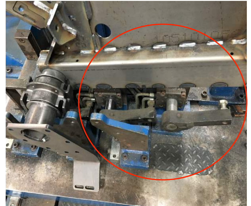
Fixture with Hydraulic Clamps
